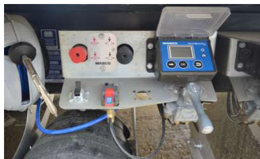
Wabco smart board for axles weight control
