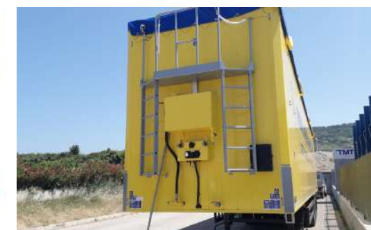
120-liters tank installed on the front of the semi-trailer
