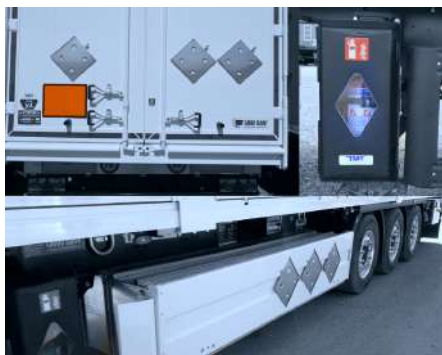
ADR kit with fire extinguisher, PVC fire extinguisher holder, neutral folding table on the rear and 3 diamond tables per side (right, left, rear)
