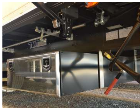
Underchassis toolbox double side openable 2400x950x380 thickness 1,5mm
